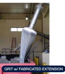
Paxxo offers custom discharge retrofit fabrication in order to mount the Longopac Fill 1H & 2V adapters to most discharges on existing equipment that is already installed in the field. Also, we now offer a dual role solution which serves as UV and wind protection. This product helps prevent the cassette bag from being blown off by the wind and is supplied with the necessary hardware to attach it to the existing discharge.
